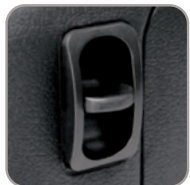
COMPRESSOR SWITCH/AIR RELEASE VALVE
